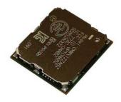
Figure 134: Module integrating a LoRaWAN stack and a LoRa transceiver
