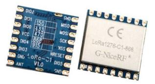
Figure 132: Example of a transceiver module (NiceRF)
