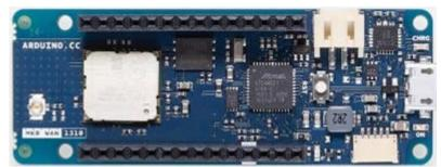
Figure 139: Arduino MKRWAN 1310: ATMEL 32 bits microcontroller + CMWX1ZZABZ Module
