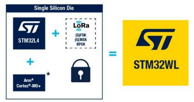
Figure 140: STM32WL dual-core microcontroller
