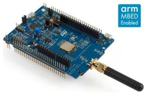
Figure 136: ST B-L072Z-LRWAN1 Discovery Board
