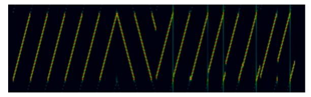
Figure 13: Spectrogram of a LoRa transmission
