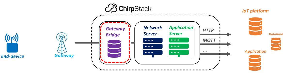
Solution 2: The Gateway Bridge handles the communication with the Gateway
